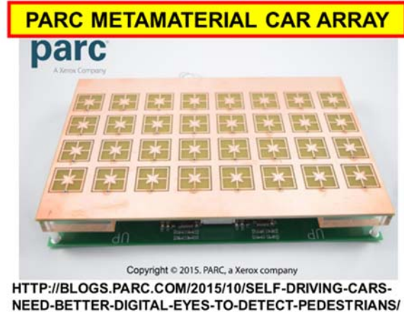
Figure 9. Metawave is developing metamaterial arrays for self driving car radars and cell phone tower usage. [18].
