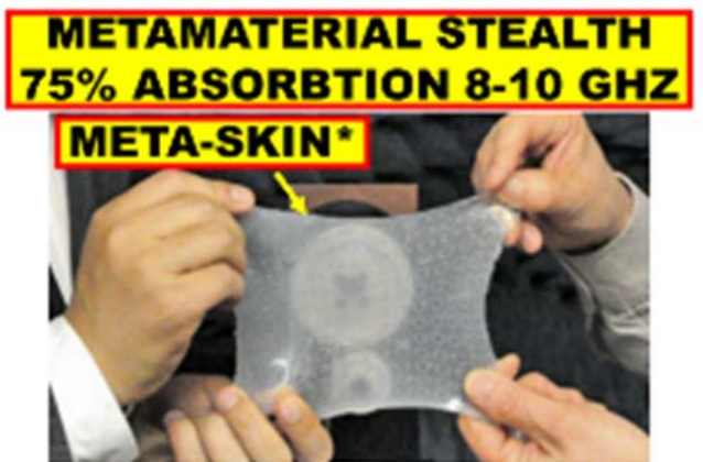
Figure 20. Stretchable, flexible metamaterial absorber [34].
